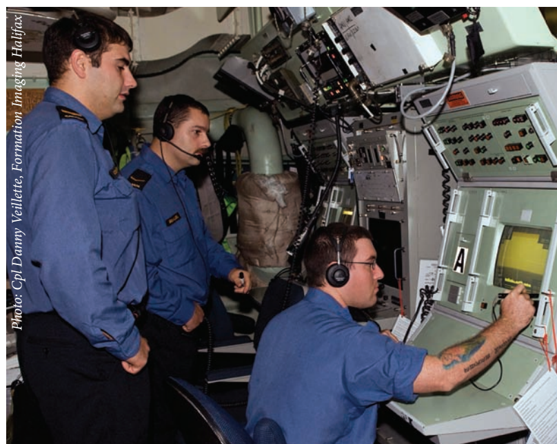
Crew members of HMCS Ville de Quebec operating the 57mm gun fire control system.
